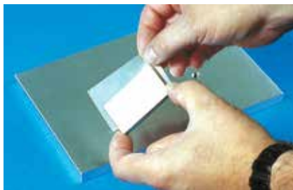
The stick form material can be used in shallow cavities for holding concave and convex pieces. It will also stabilize delicate parts during machining.
