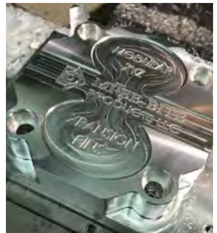
Op 2 including c'bore on same fixture
